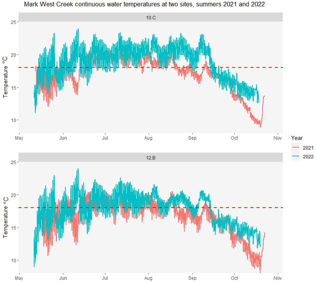
Figure 40. Mark West Creek continuous water temperatures at sites 10.C (top panel) and 12.B (bottom panel), summers 2021 and 2022. Dashed red line represents 18 °C avoidance threshold.
