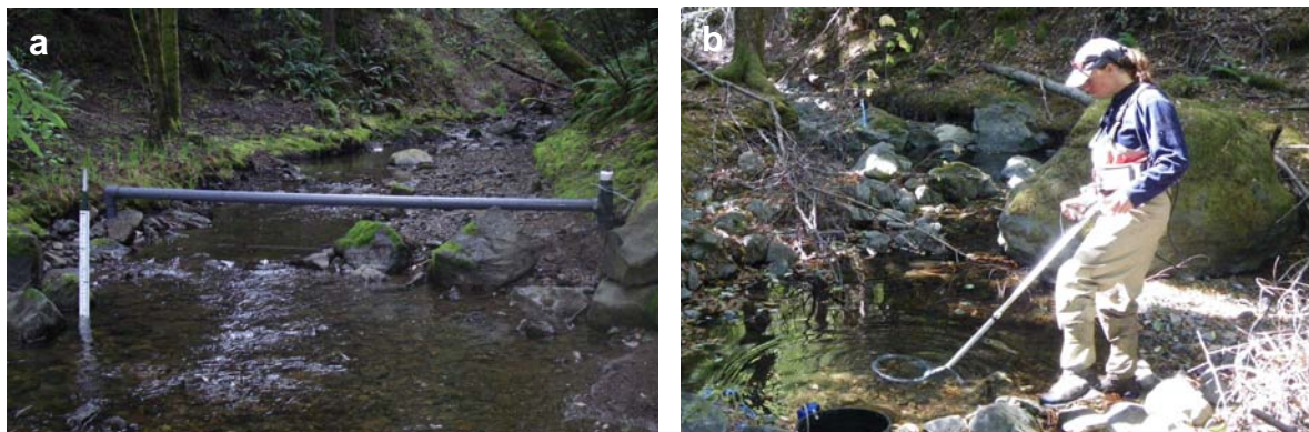
Figure 2. Stationary (a) and portable (b) PIT tag detection systems used to detect movement and presence of PIT tagged coho in Mill and Palmer study reaches.
